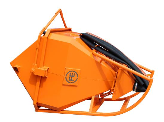
The CS1034C range of Column Skips, have been specifically designed by the manufacturer Eichinger to meet the specific needs of pouring concrete into columns and formwork. With the delivery hose attached to the gate of the skip users can direct the flowing concrete with ease.
