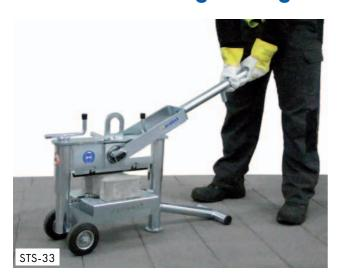
The combination of lever/eccentric transmission and the special triangular knife produces an enormous splitting force – with minimal use of force.
