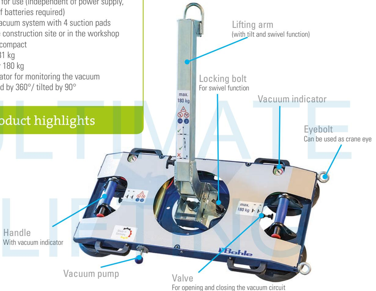
The manual lifting device can do without an electric pump and is therefore very versatile in use. A dual circuit vacuum system, reserve tanks, vacuum display and an additional visual vacuum indicator ensure high levels of safety. The manual lifting device stands out due to its very compact construction and low weight.
